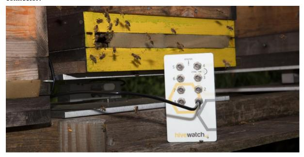
Properly aligned, the four-pin connector is easily inserted and the sleeve tightened with little resistance. As this is an extremely accurate measuring system, it is important that the contacts do not become contaminated or come into contact with water. Installation should be carried out in good weather to ensure that no moisture, dust or dirt enters the connectors.
