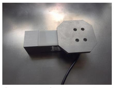
After correct positioning of the spacers, the top and bottom plates must be set in place such that the load cell is correctly centred between them and then secured with the mounting screws provided. To ensure maximum platform stability, these must be thoroughly tightened. After initial attachment of the top and bottom plates and hand-tightening of all eight screws, the fasteners must then be drawn fully tight. The scale
